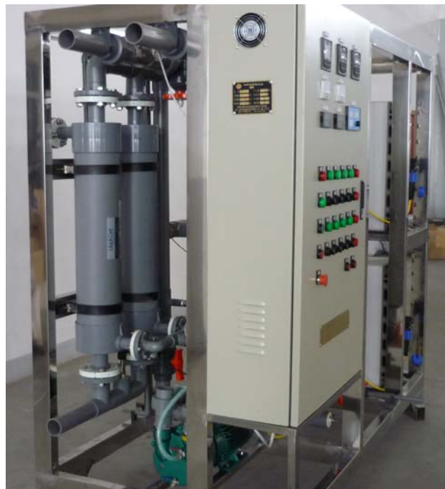
6-inch Liqui-Cel® Membrane Contactor System Upstream of EDI
