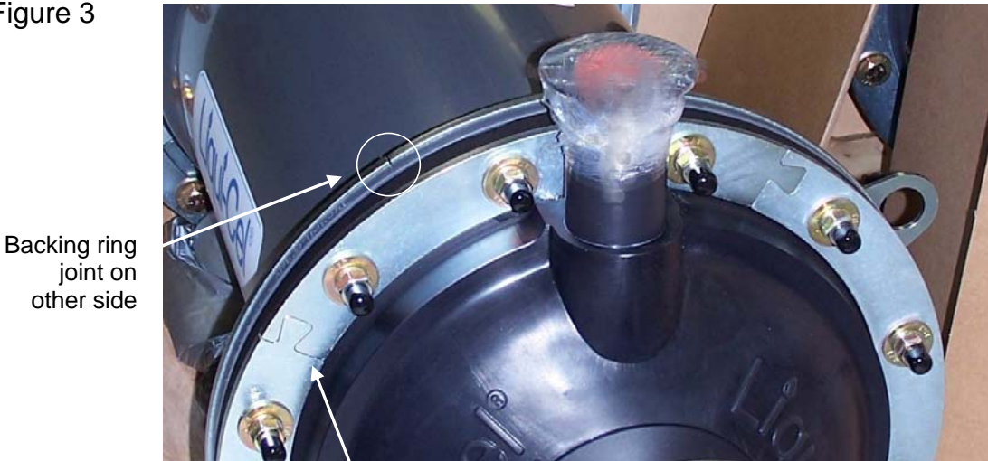
Backing ring joint on this side
